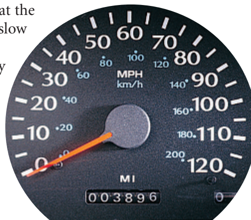
FIGURE 4.4 ▲ The speedometer for a North American car gives readings of instantaneous speed in both mi/h and km/h. Odometers for the U.S. market give readings in miles; those for the Canadian market give readings in kilometers.
