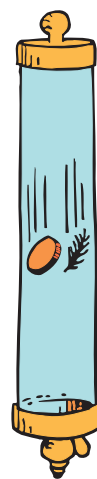
FIGURE 4.13 ▲ A feather and a coin accelerate equally when there is no air around them.
